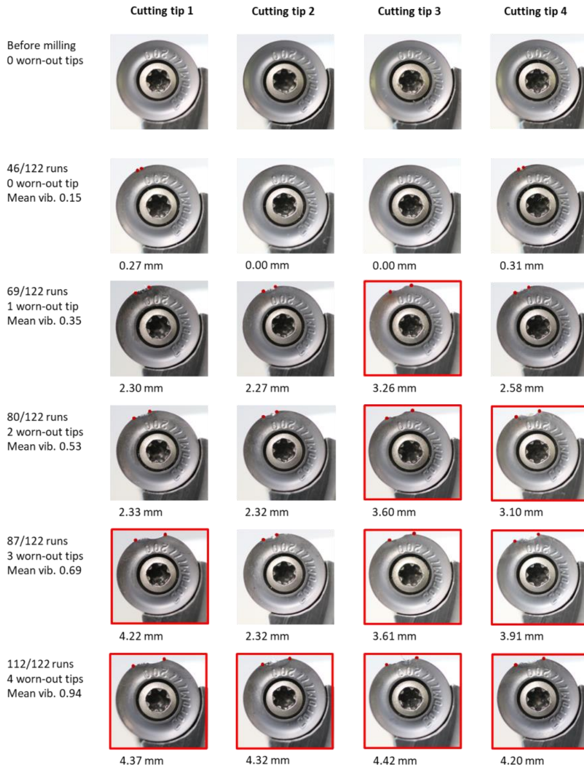
Figure 3: Example for evaluation of functional state of cutting tips within one milling cycle. The cutting tip was regarded worn-out and insufficient as soon as the break-off edge was longer than 3.1 mm and exceeded the maximum point of the cutting sector (marked by red border). The mean vibration value was calculated for each stage with the respective number of insufficient and worn-out cutting tips.
