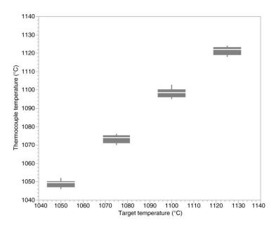
**Figure 2:** Boxplot diagram showing the temperature of the melt as measured by thermocouple for four different target temperatures (1050°C, 1075°C, 1100°C and 1125°C).
