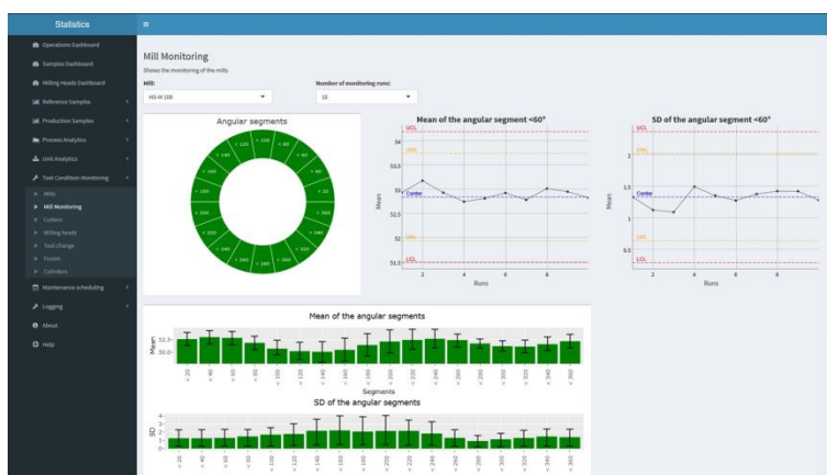
Figure 4: Dashboard of the PM Analytics used for TCM of the swing aggregate. For detection of deviations methods of statistical process control (SPC) are applied.
