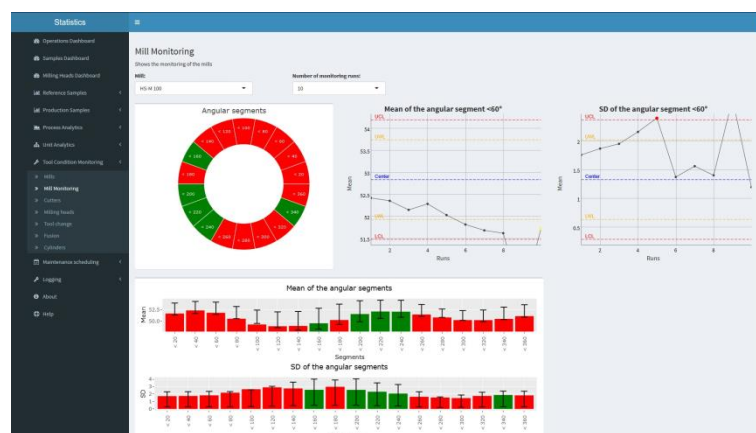
Figure 5: Example of a dashboard showing the typical pattern of a worn grinding set.
