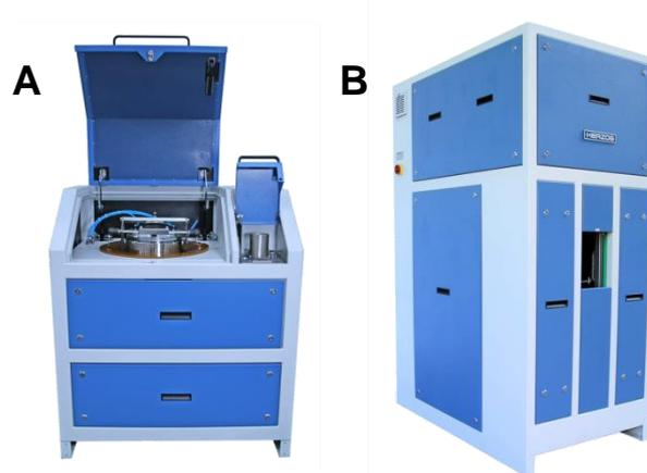
**Figure 1:** (A) Manual pulverizer HP-M 500. The grinding vessel needs to be filled, cleared and cleaned by the operator.
