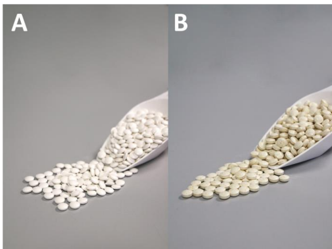
Figure 1: Photographs of the grinding aids of (A) the type HMPA 40 (MCC) and (B) the type HMPA 100 (pine resins)
