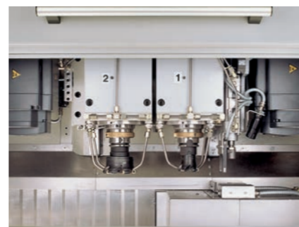
Two independently operated precision milling spindles can be fitted with milling cutters for various material grades.
