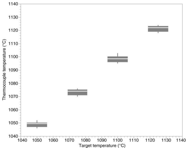
**Figure 2:** Boxplot diagram showing the temperature of the melt as measured by thermocouple for four different target temperatures (1050°C, 1075°C, 1100°C and 1125°C).
