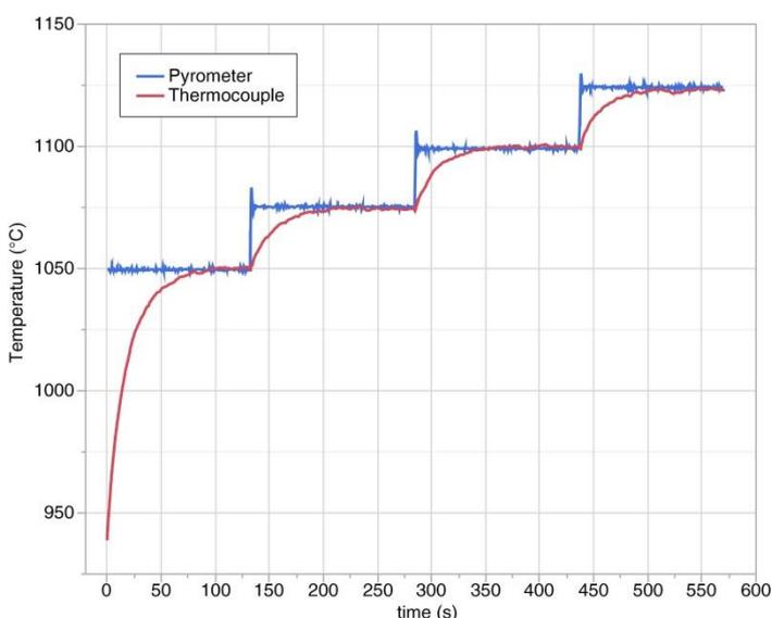
**Figure 1:** Example for evaluation of the deviation of the melt temperature (measured by thermocouple, red) from the target temperature (measured by pyrometer, blue). Four temperature stages (1050°C, 1075°C, 1100°C, 1125°C) were assessed subsequently.
