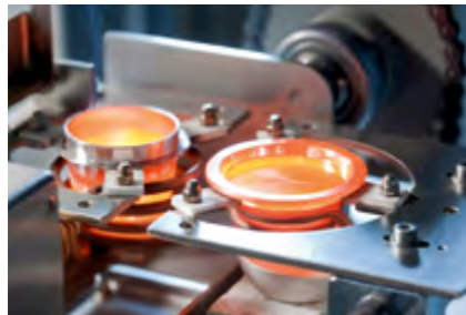
Operating sequence in the fusion module with induction heating in the crucible, ...
