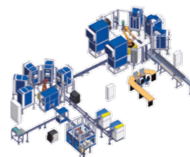
Assmang Automatic laboratory for iron ore (Khumani Mine, South Africa)
