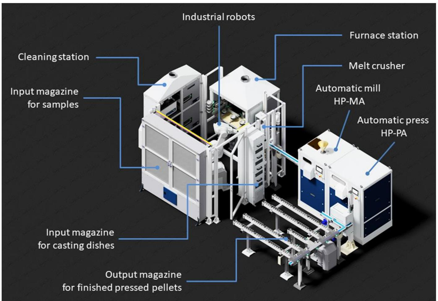
**Figure 1:** Layout of the automated system for pyrosulfate fusion, crushing, pulverizing and pelletizing of sample material. A further component of the automation is the cleaning station for ultrasonic cleaning and hot air drying of the crucibles containing solidified rest material after fusion.
