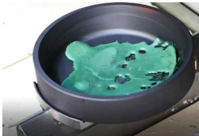
**Figure 3:** Casting dishes are designed to allow quick cooling and prevent sticking to the wall.
