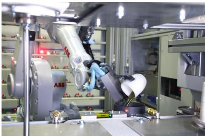
**Figure 2:** Pouring of the melt from the crucible into the casting dish by the multi-axis robot .
