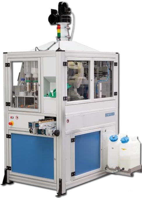
**Figure 1:** Automatic high-frequency fusion system model HAG-HF (Herzog, Germany).
