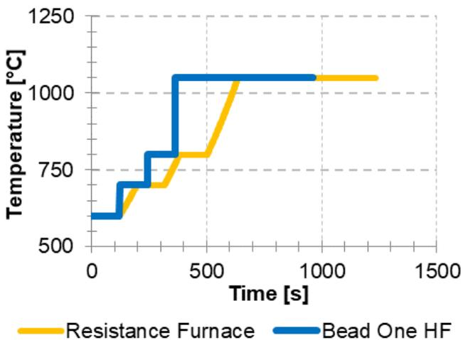
**Figure 2:** Heating profile of the Bead One HF in comparison to a resistance furnace. It is also possible for the Bead One HF to set ramps with different slopes in order to slow down the heating.
