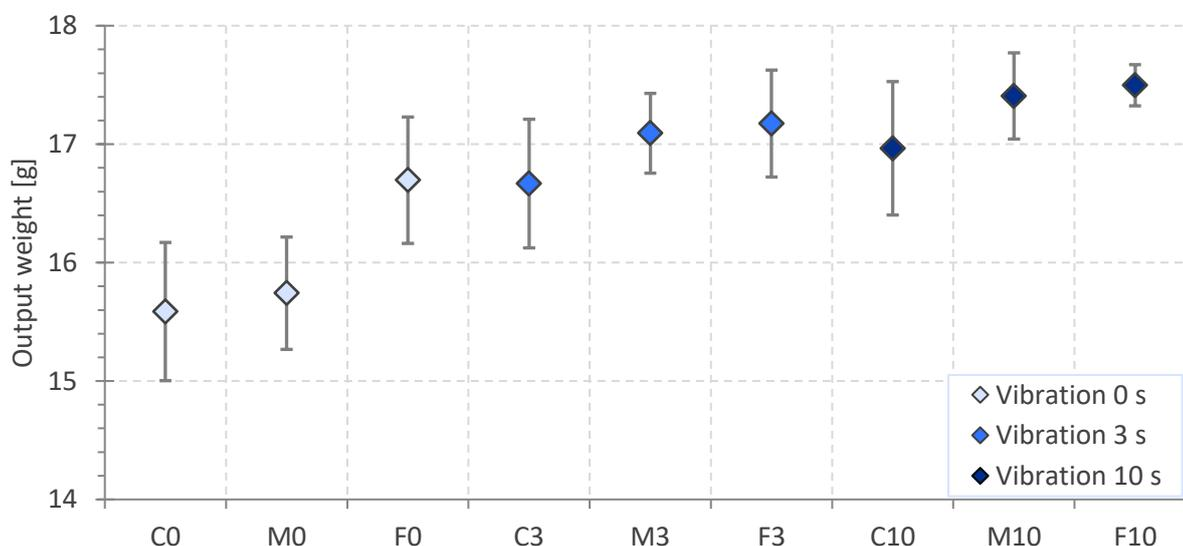
**Figure 1:** Output weight of ground clinker for the nine different conditions. The conditions are sorted according to the applied vibration time of the dosing spoon from no vibration, 3 s vibration to 10 s vibration.
