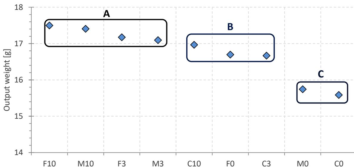
**Figure 2:** Arrangement of conditions into homogeneous groups, which do not differ statistically in terms of output weight. Especially group C showed significantly lower output weights than the other conditions.
