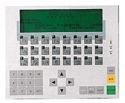
Storable parameter programming via the operator terminal, protected by password, for fully automated operating cycles and precise reproducibility.
