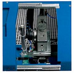
The easily accessible sample holder with pneumatic clamping unit guarantees reliable, defined gripping.
