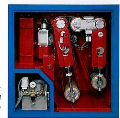
also allows the grinding belt and milling cutter to be used not only in combination but also for separate grinding and milling operations.
