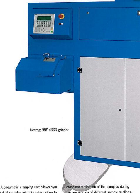
metrical samples with diameters of up to 60 mm to be gripped reliably and in a defined position, thus enabling high grinding and milling capacities and short sample preparation times.
