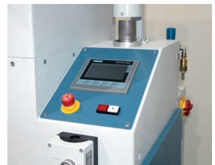
HMI panel of the manual HUST
