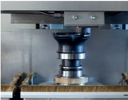
Milling of samples takes place from below for extremely fast sample handling
